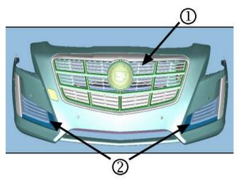
**Note:** For vehicles with bright chrome grille kits, replace the upper grille (1) and front outer grilles and bezels (2) with the black chrome service parts noted above. For vehicles with black chrome grille kits, replace ONLY the front outer grilles and bezels (2) with the service parts noted above.
