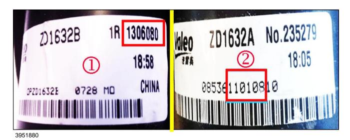
**Example (1):** The date is the first six digits in the top corner of the label. The date on the motor in this example is 130608, which is June 08, 2013 (AFFECTED).
