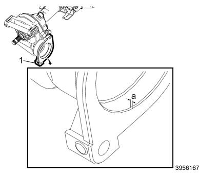
**Caution:** First design steering motor with a small chamfer does not require a seal. If a seal is installed on a first design steering motor, potential damage to the steering motor may occur resulting in loss of assist steering. Seal is only required for the second design steering motor with the larger chamfer. Before installing the power steering assist motor, inspect the power steering assist motor housing (1) to verify the steering column design.
