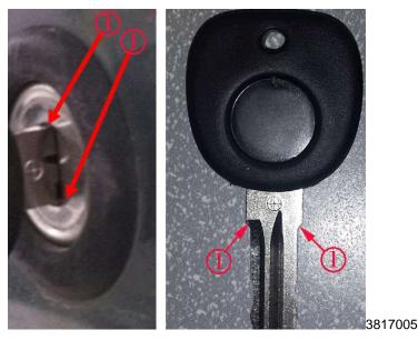
**Note:** Without the modification, the key stops on the shoulder and will not fully enter the key lock cylinder. Refer to the photograph.
