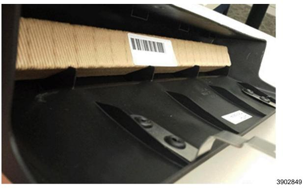
3.1 Install the energy absorbing material into the brow so that the barcode is facing towards you and is resting on the four angled ribs.
