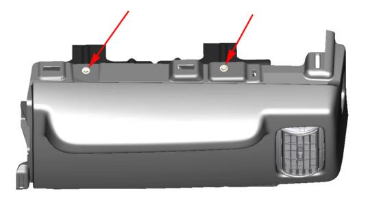
2. Remove the upper two screws that attach the instrument panel pad to the instrument panel bracket.
