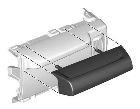
4. Install the brow assembly to the instrument panel.
