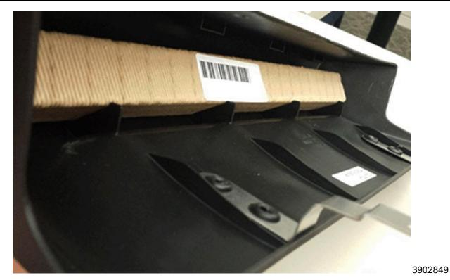
3.1 Install the energy absorbing material into the brow so that the barcode is facing toward you and is resting on the four angled ribs.
