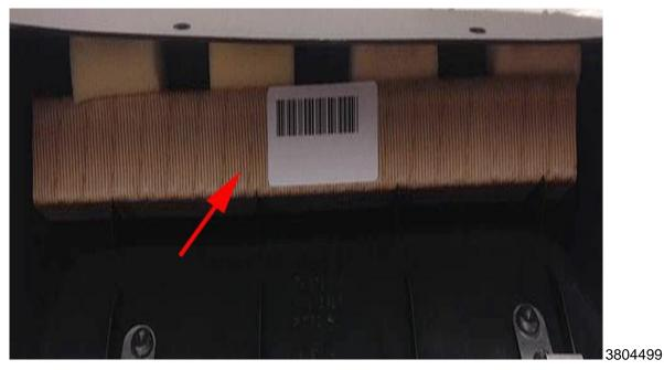
3. Inspect the brow assembly before installation to ensure the energy absorbing material is present.
