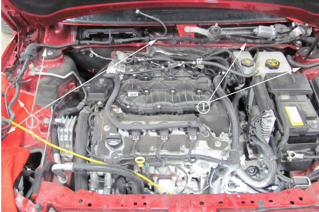
View of the forward lamp harness (1) with the required parts removed from the vehicle. Do NOT begin removing the harness until the required parts have been removed.
