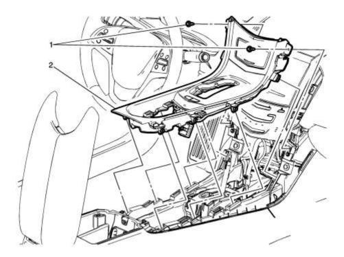
2. Remove the front floor console trim plate (ATS vehicles). Refer to *Front Floor Console Trim Plate Replacement* in SI. Remove the Front Floor Console (CTS vehicles). Refer to *Front Floor Console Replacement* in SI.
