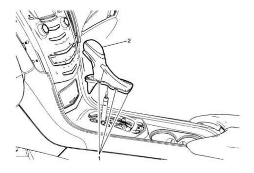
8. Install the transmission control lever knob for automatic transmission. Refer to <u>Transmission Control Lever Knob Replacement</u> in SI
