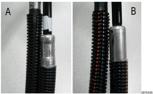
(A) Crimped ferrule with swedge marks. This is a secure connection on the pipe ferrule. (B) Uncrimped ferrule without swedge marks. This is NOT a secure connection on the pipe ferrule.
