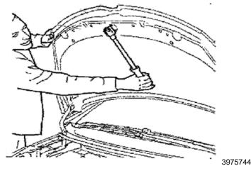
3. Apply 72 Nm (53 lb ft.) of torque to the striker while holding the hood with the opposite hand.
