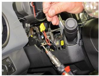
**Warning:** DO NOT use soldering equipment that is battery or electric powered. These types of soldering irons can induce voltage into the circuit, which may cause damage to electrical components. Use only the J-38125-5A Ultra Torch or another butane fueled soldering iron when working on SIR circuits.
