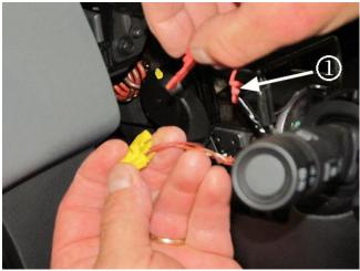
2. Remove the CPA (1) from the air bag coil X2 connector.
