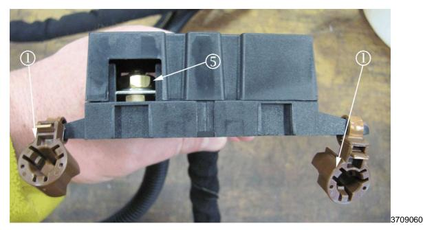
• A fuse block housing assembly that has NOT been reworked will have two brown clips (1) that secure the fuse block housing assembly to the shock tower studs. The fuse block housing cover will also NOT have a black polyolefin side window shield (5) or a black polyolefin bottom shield that is secured to the fuse block housing assembly with two black tie straps. If the fuse block housing assembly rework has NOT been performed, perform the rework procedure in this bulletin. Proceed to step 3.
