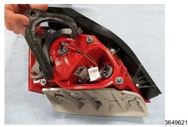
4. Slowly peel the seal away from the housing, using care to remove the adhesive from the housing. **Tip:** Removing the seal at a 45 degree angle while slightly stretching the rubber will remove most of the adhesive with the seal.
