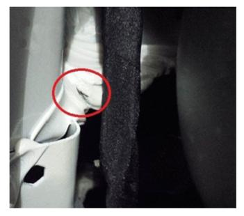
2. Inspect for voids in the body sealer at the cowl seam on the left side as in picture below
