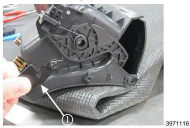
6. Install the new replacement inertia latch and spring assembly (1) to the compartment.
