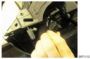
6.2 Slide and install the inertia latch onto the compartment. Push in the pivot pin to snap the latch into position.
