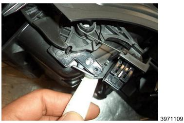
5.1 Using a trim stick, or suitable tool, push the inertia latch pivot pin out from the bottom.
