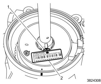
3. Document the last 9 digits of the NEW steering shaft torque sensor on the vehicle repair order. The serial number is located on the bottom of the caution label (2).
