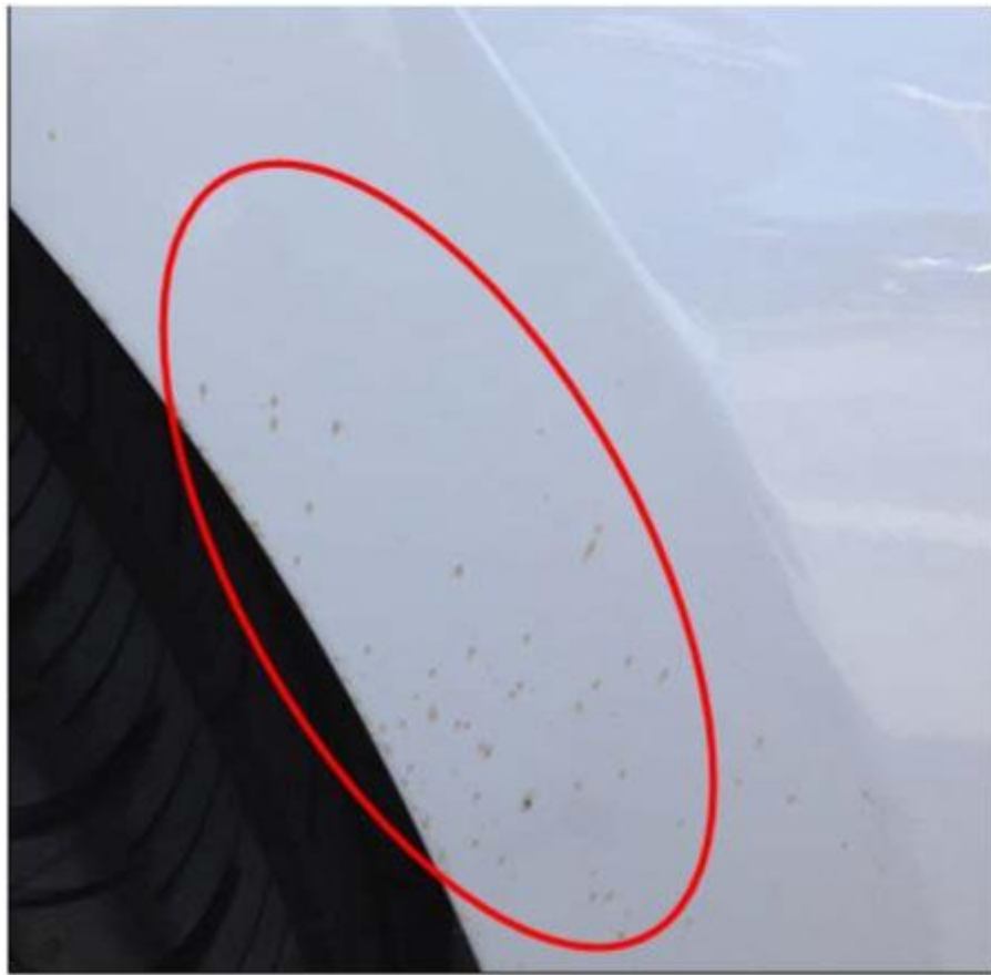
Figure 2. Paint damage due to slinging tire dressing residue.
