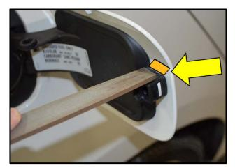
⇐ Install protective tape on fuel door in marked area <rectangle>, then using a flat file (or equivalent), remove the excess material from the fuel door latch as shown <arrow>.
