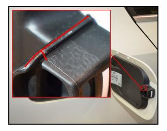
Tip: Excess material and burrs may be present along the ridge of the housing where the plastic seams join together as shown <red lines>.
