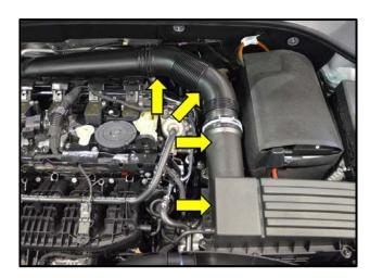
Remove the air filter housing and intake tube <arrows>.
