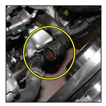
Disconnect the heater core hose from the "Y" connection near the driver side cooling fan <circle>.
