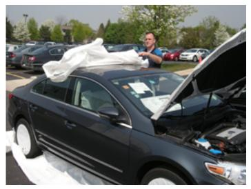
• Cut the upper FBC around the windshield and roll cover towards rear of vehicle.
