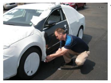
• Remove clips and hooks under the rocker panel.
