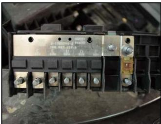
⇐ Using a pocket screwdriver, or equivalent, gently pry the SA portion of the fuse panel off the old fuse panel <arrow>.
