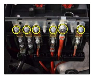
Section D – Fuse and Fuse Panel Replacement
