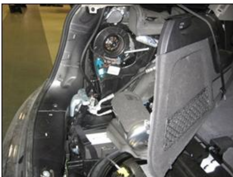
Figure 9. Location of rear air conditioning unit and expansion valve.
