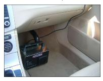
8. Route the cable of cleaner through the side window to the outside. Close the side window and connect the power cable. A self-test starts; when a green arrow lights up the unit is operational.
