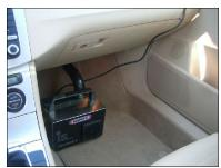
8. Route the cable of cleaner through the side window to the outside. Close the side window and connect the power cable. A self-test starts; when a green arrow lights up the unit is operational.
