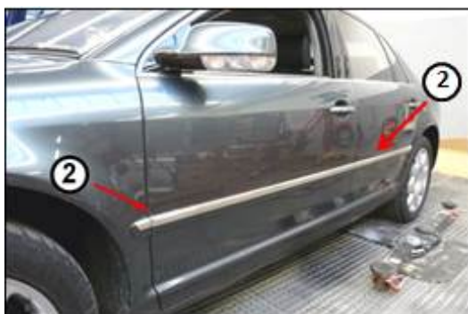
Figure 2 – Central protective strip
