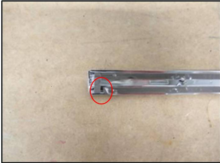
Figure 2 (the red circle shows the opening of the incomplete bonding)
