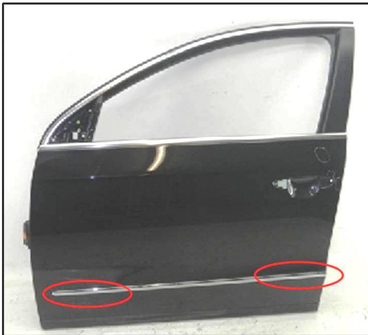
Figure 1 (the red ellipses show the area which can be affected by the corrosion)
