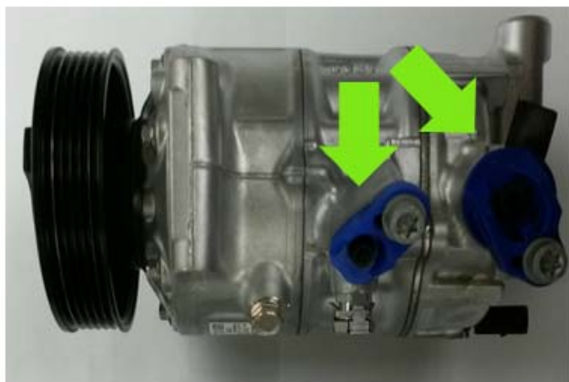
A/ C Compressor
