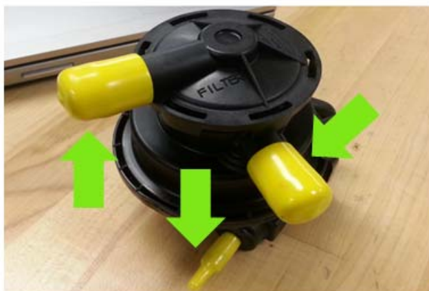
Leak Detection Pump
