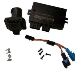
5N0 055 204 N – Trailer Hitch Electrical Kit
