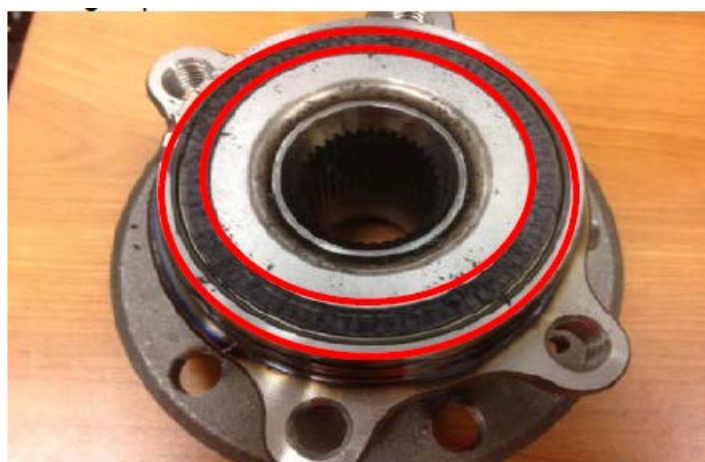
Encoder Ring Destroyed
