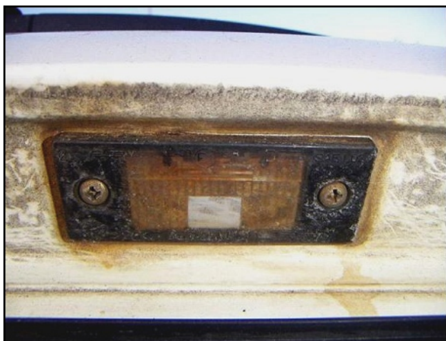
Figure 1: corrosion on and around the license plate light - example 1K5, screw installation
