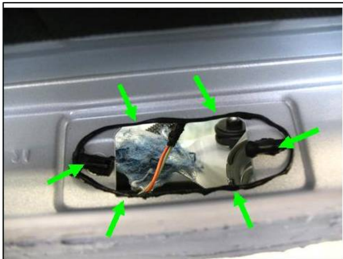
Figure 5) example 1K5 –License plate light, contact surface and hole sealed with butyl sealing cord
