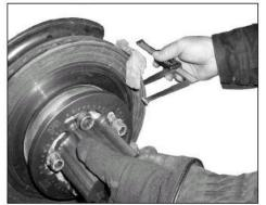
Technician must record the final thickness measurements on the back of the repair order.
