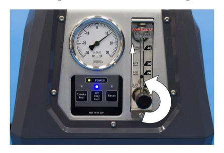
Block the pressure output hose with your thumb until the pressure gauge displays approximately 12 in.H<sub>2</sub>O.
