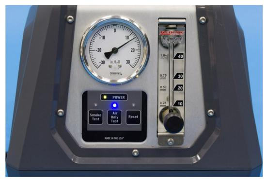
If a leak is suspected, press the Smoke Test button and allow the system to fill with smoke. Visually inspect the system for signs leaks with the aid of the Halogen Inspection Light. Adjusting the Flow Control Knob may assist in pinpointing a smaller leak.
