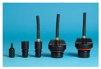
The filler cap adapters provide a pressurization input for the Subaru Portable Leak Detector. The two filler cap adapters appear very similar. Using the wrong adapter may cause a leak or damage the adapter or filler neck. The dual start adapter is labeled. The single start adapter is not labeled. Perform a check on the gas cap of the test vehicle by rotating it by 180 degrees to see if there is two thread starts or a single start. Select the matching filler cap adapter.
