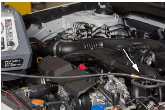
**NOTE:** If the ELCM is pressurized from the drain outlet, some leakage from the ELCM's waterproof electrical connector may occur. This is normal, as the drain side of the ELCM is normally only exposed to atmospheric pressures. So, any pressure greater than atmospheric pressure can induce leakage.
