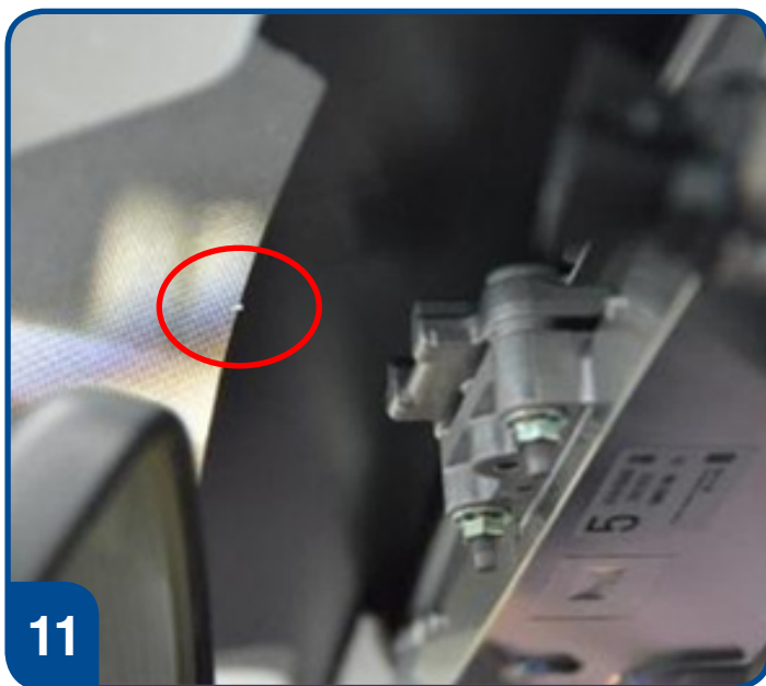
Locate the windshield upper shade center mark to align the mirror harness and cover
