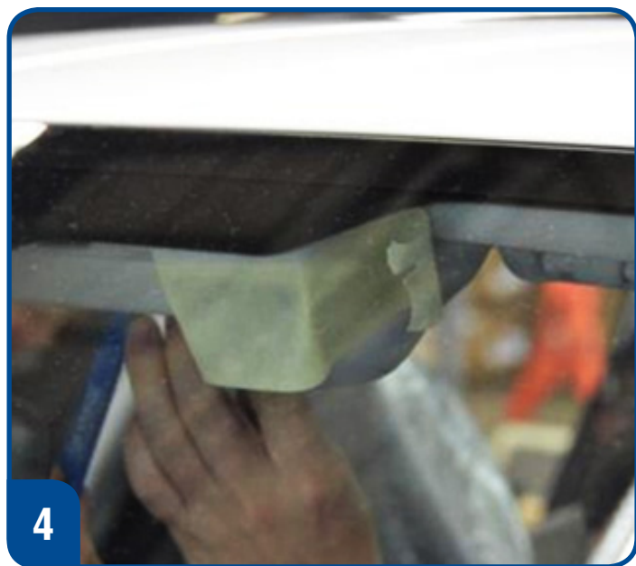
Apply protective tape to the eye sight camera openings. DO NOT TOUCH THE LENSES
