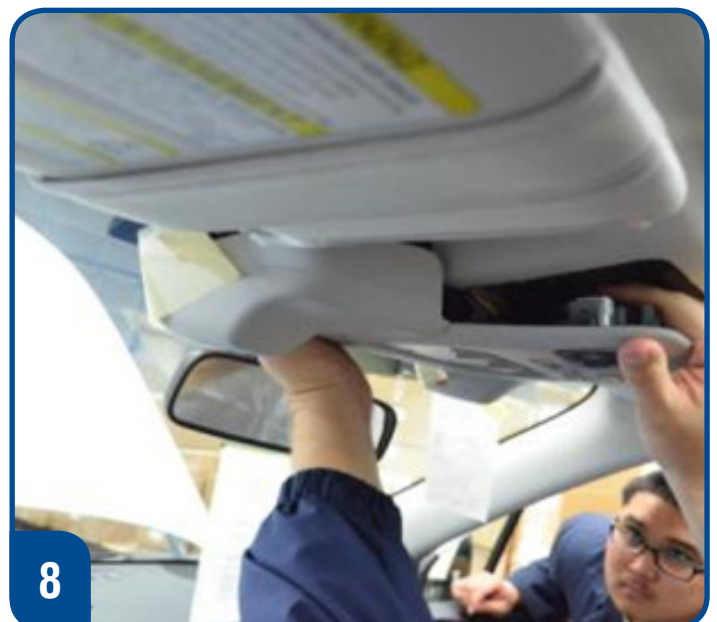
Carefully pull down on the cover from the headliner to remove the cover from the headliner. Support the front of the cover when removing.
