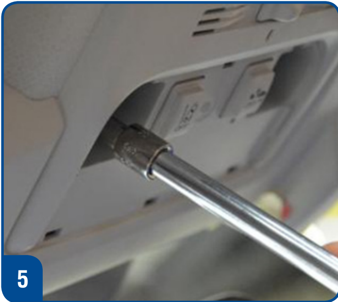
Using a 8mm socket remove the Eye Sight cover retaining bolts (2)
