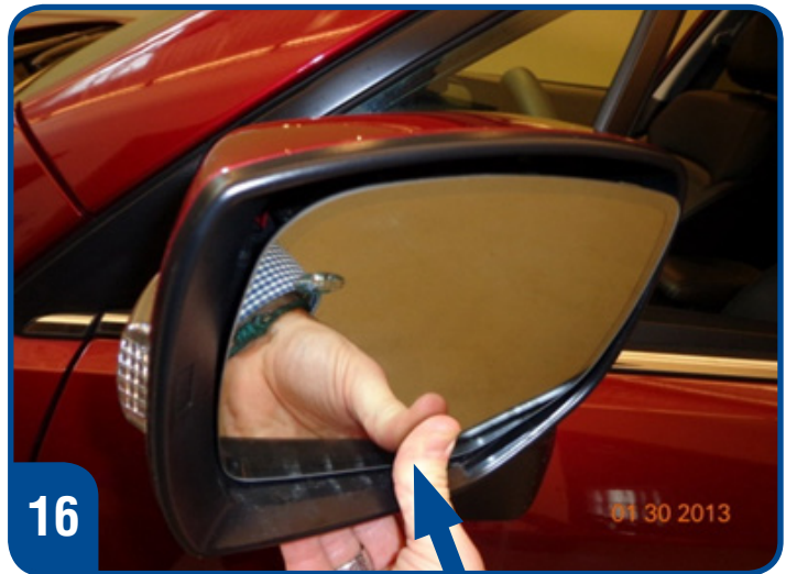
16 Press Down to Snap & Lock
