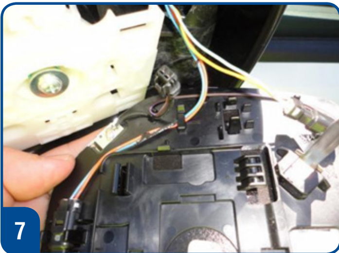
7 Route lower harness through under side clip.
