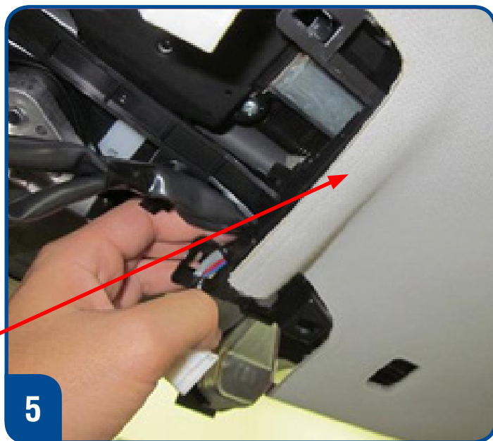
Carefully access the connector without damaging the headliner
