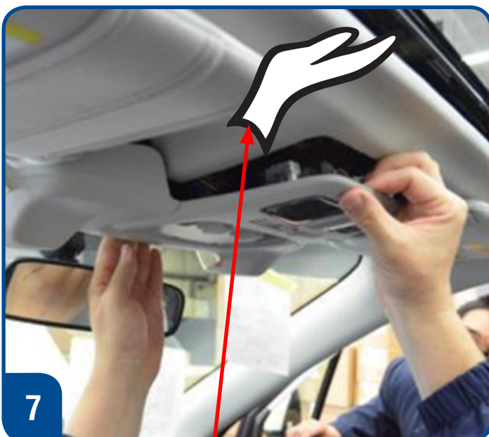
Carefully support the headliner here when pulling down on the cover.
