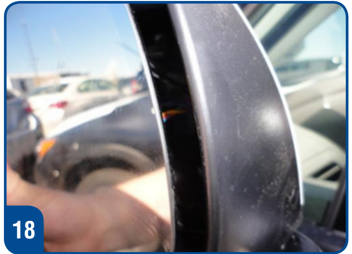
Harness stays back though mirror's entire range of motion.
