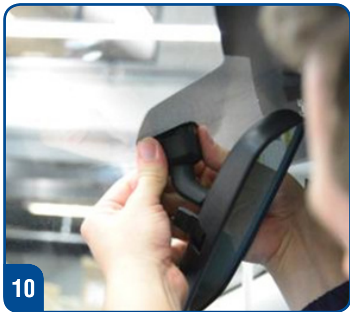
Remove the original mirror
