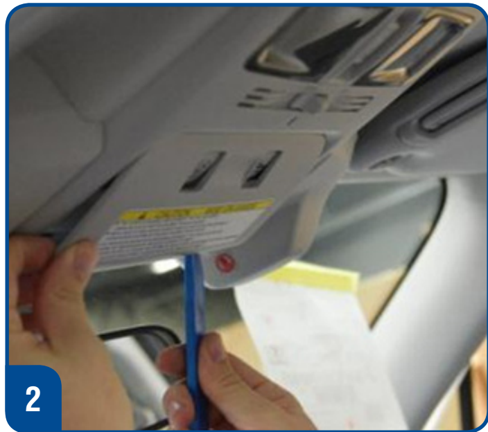
Carefully Pry off the Cover
