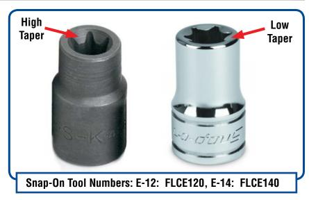
assistance in locating one of each size of these special sockets. As shown in the photos above, there are differences in the "taper" areas of these sockets. Be sure to specify that you need a "low taper" or shallow counter-sunk socket for this application.
