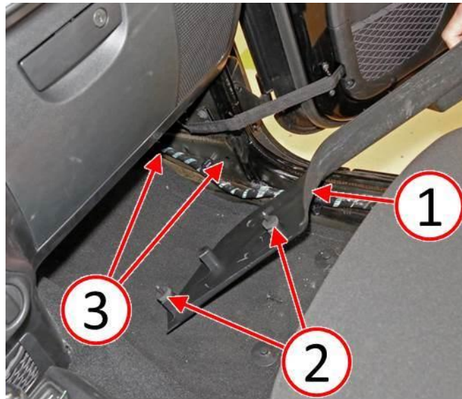
Fig. 2 Remove Cowl Trim Panel
