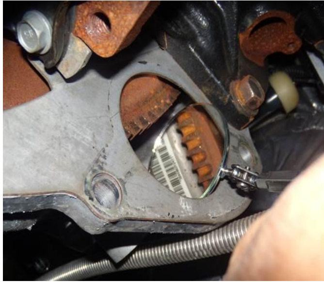
Fig. 2 Torque Converter Label Inspection
