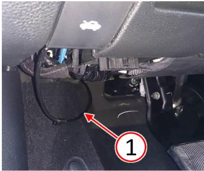
Fig. 1 Hood Release Cable Hanging Down
