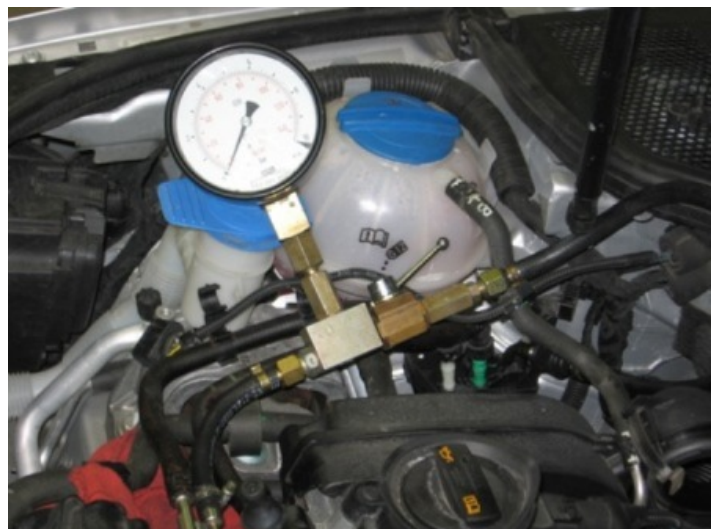
Figure 1. Measuring low-side fuel pressure with VAG 1318 gauge.
