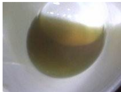
Figure 1. Fluid photograph example showing approximately one inch of fluid in the white cup, and tilted on an angle to show depth and color.
