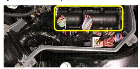
Figure 5. Engine control module (ECM).
