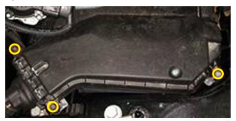
Figure 4. Screws to be removed (outlined).
