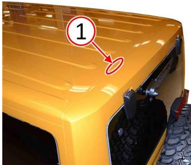
Fig. 1 Area Of Leak Concern
