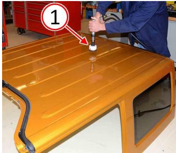
Fig. 5 Destroy Defective Hard Top To Prevent Reuse
