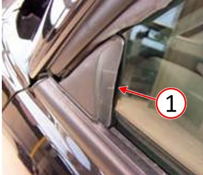
Fig. 1 Window Flag Gap Inspection
