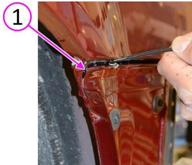
Fig. 3 Apply Sealer Into Back Of Slot
