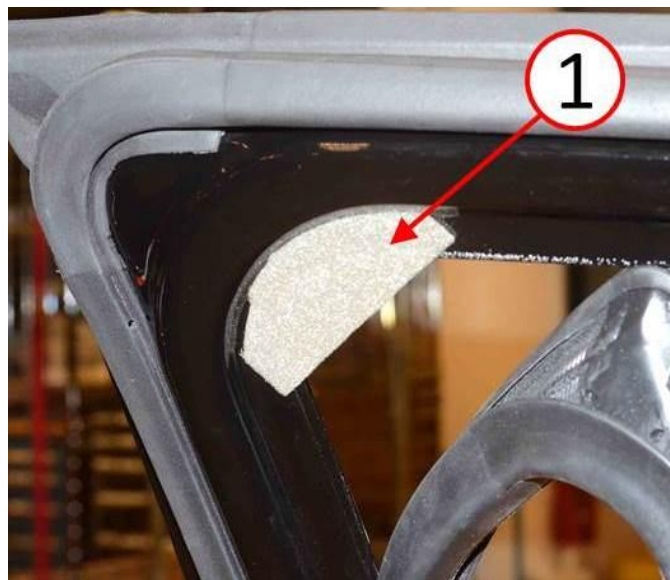
Fig. 3 Foam Piece Installed
