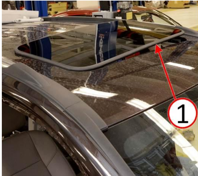
Fig. 7 Sunroof Glass Panel Installation
