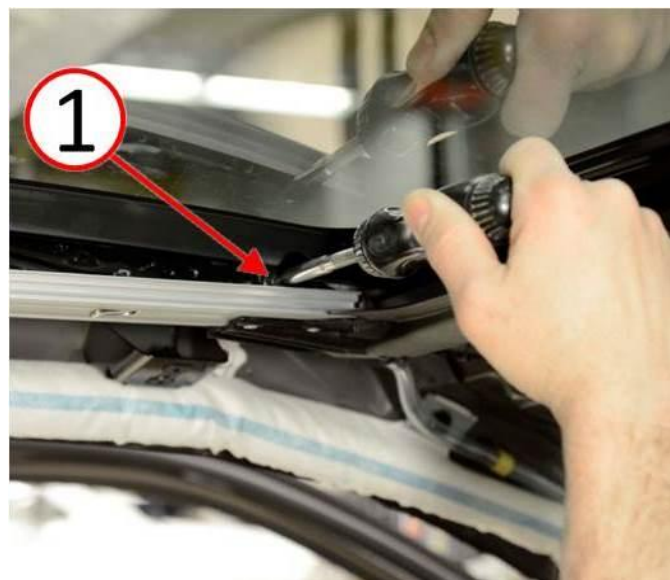
Fig. 11 Sunroof Glass Panel Set Screw
