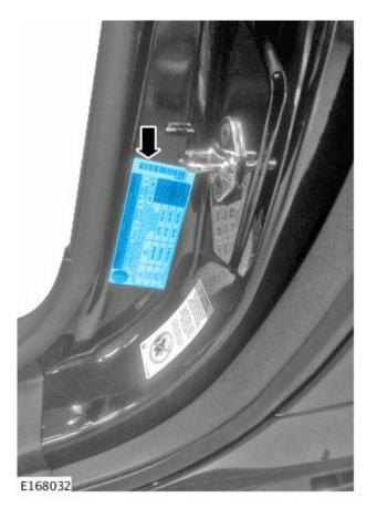
6. NOTE: Make sure there are no air bubbles or debris under the label and the body surface is clean.
