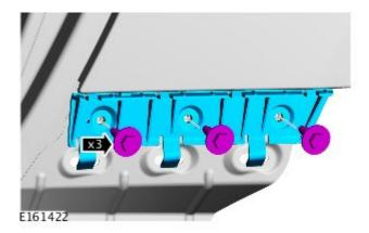
5. Remove the rocker panel moulding bracket.
