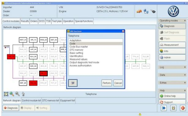
**Step 4)** Select network diagram, double click the Red TEL 77 icon, select Control module OBD, Select Code and press perform.
