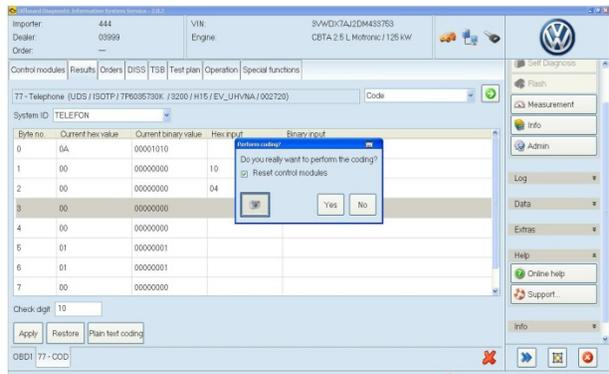
**Step 6)** New coding should be 0A 10 04 00 00 01 01 00. Once the new values are entered select Yes to perform coding
