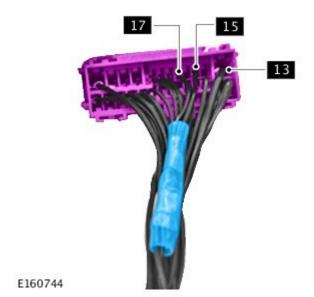
**6.** If necessary, repeat step 5 to the front left door electrical connector (C3A-C2).
